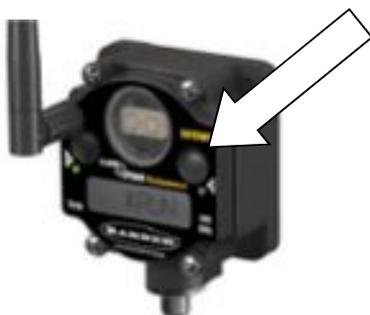
Push button 2 for binding to field radios.
