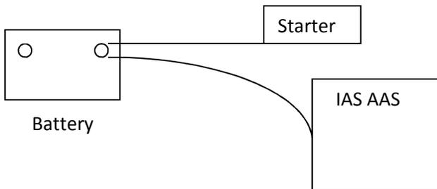
You need to connect the 12 gauge wire from the battery posts directly to the IAS AAS charge controller positive and negative terminals as shown on the following page. See document 6 for the detail AAS wiring diagram.
