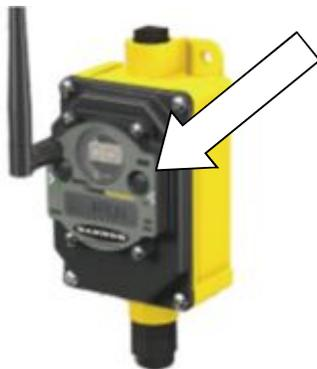
Push button 2 for binding to field radios.
