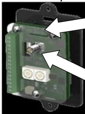
Push button for binding to field radio's.
